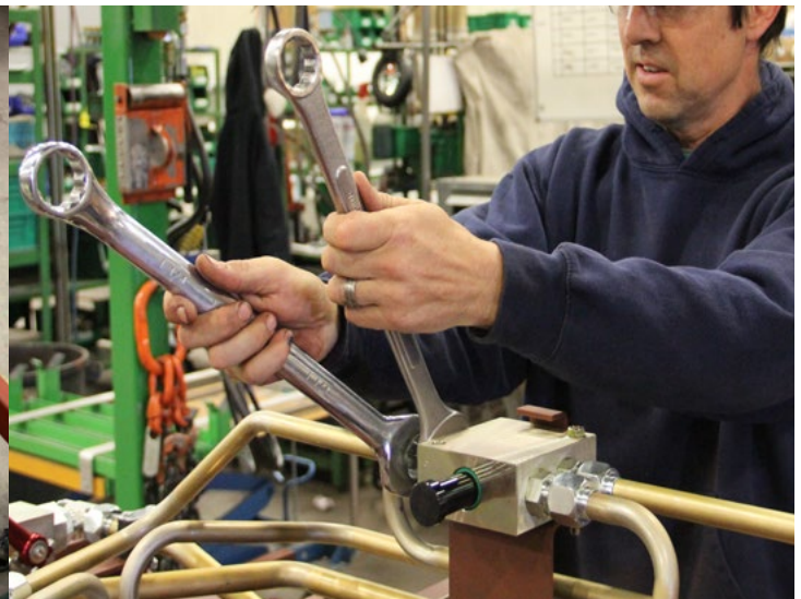
•At Control Valve end, loosen fitting using 1-1/8" wrench and a 1-1/4" wrench.
