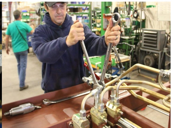
•At Check Valve end, loosen fitting connecting the Front of Cylinder #3 to Control Valve using 1-1/8" wrench and a 1-1/4" wrench.
